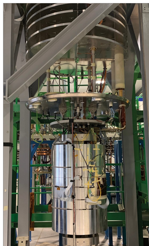
A Nb 3 Sn demonstrator racetrack dipole magnet with no bore developed at CERN in the framework of the Future Circular Collider study, which reached a record peak field of 16.5 T in February. Photo: J Perez/CERN
