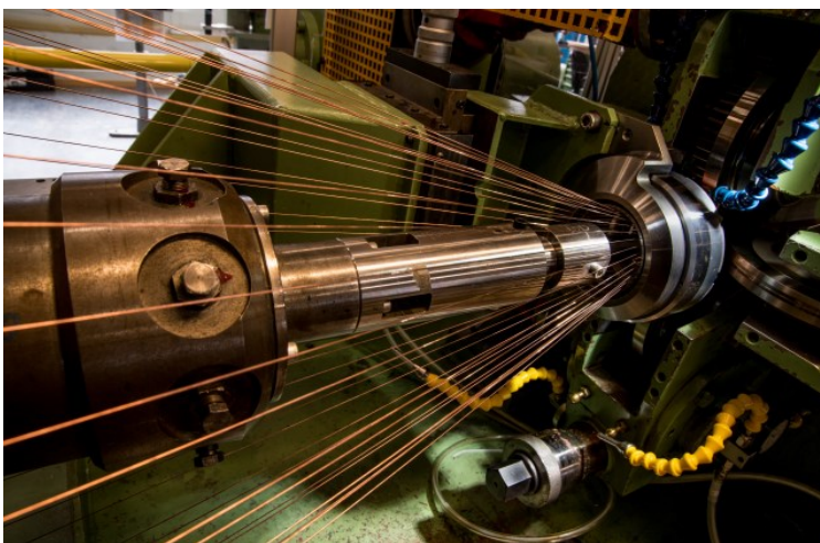
A Rutherford cabling machine is used to assemble the high-performance cables, made from state-of-the-art \text{Nb}_3\text{Sn} conductor, for the LHC High Luminosity upgrade. (Photo: Max Brice/CERN)
