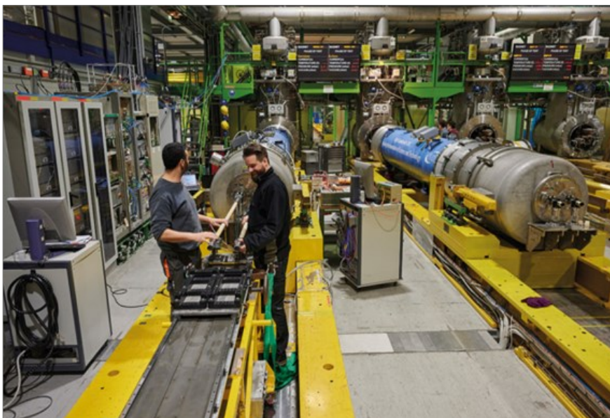
Power couple \text{Nb}_3\text{Sn} 11 T dipoles for the HL-LHC undergoing tests at CERN's SM18 facility in February. Photo: CERN-PHOTO-202002-038-5
