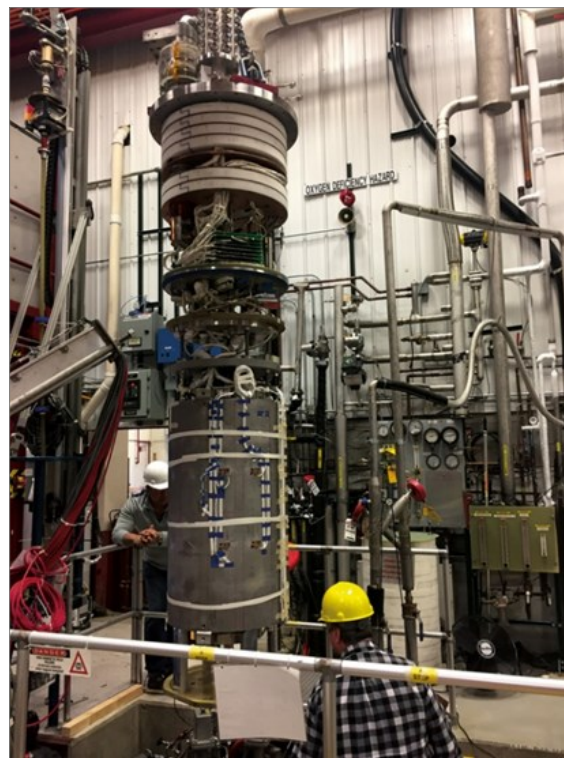
The MDP “cos-theta 1” dipole accelerator magnet at Fermilab, which achieved a field of 14.1 T (the highest ever achieved for such a device at an operational temperature of 4.5 K) in 2019.
